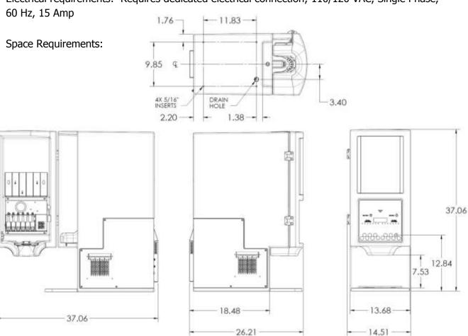
Note: Please allow an additional 6" clearance behind the unit to facilitate proper cooling and air circulation.
